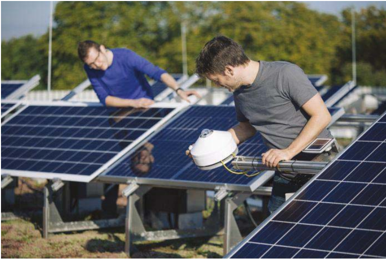
Figure 2. Pyranometers, such as the plane-of-array sensor shown here, require periodic calibration to maintain their accuracy. What is unknown, however, is how local climatic factors affect calibration drift and therefore how much measurement uncertainty exists across different operating environments.
